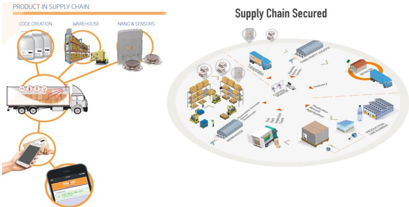
During the manufacturing process, unique codes are applied on each pack, carton and master case and are subsequently scanned. It enables each packaging unit to be tracked along the supply chain without the need for unpacking, scanning and repackaging of each unit. At the backend, each MultiSense is interlinked to a specific box and the box is interlinked to its content. As products travel the supply chain, movements are scanned by warehouse operators and the journey history recorded.
