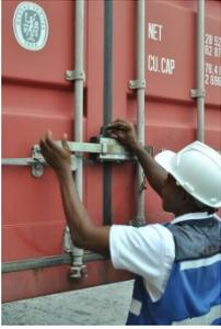
After many failures and lots of resources spent, the **CelloTrack Container Lock** proved to be the best solution available in the market. CelloTrack's IP67 standard, huge battery capacity and robust specifications made it a unique alternative for our application needs.
